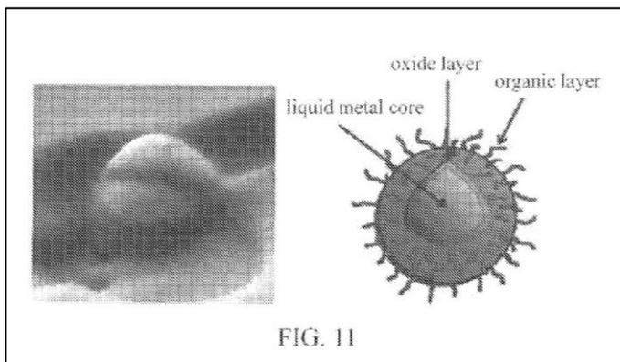
An SEM image and a schematic of an etched core-shell particle in accordance with this invention.
